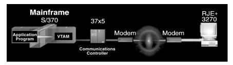
A PC running Barr 3270 software replaces a cluster controller and attached 3270 terminals.
