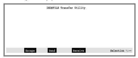
The options on the bottom of the screen display each time the File Transfer utility is selected and after each send or receive transfer.
